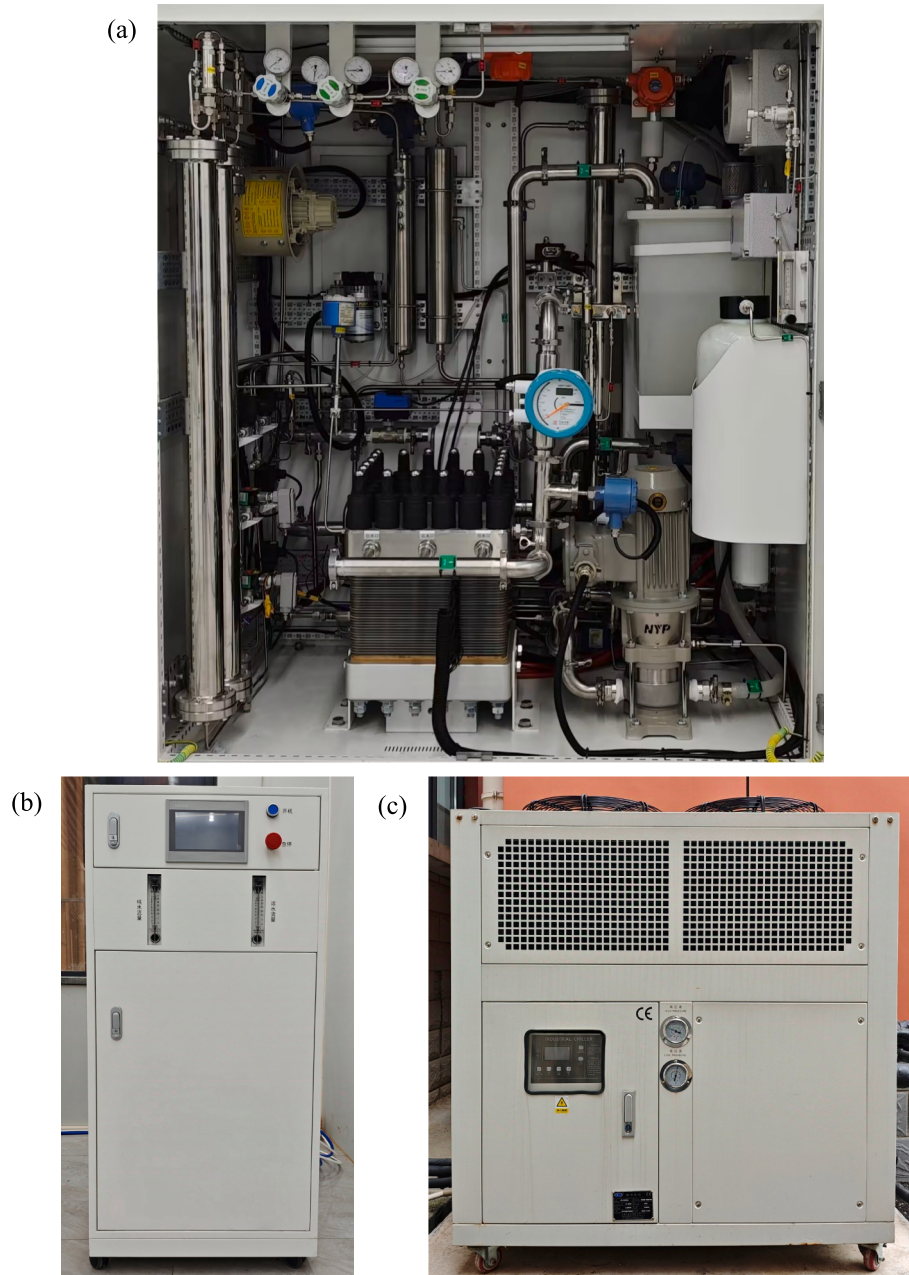
Fig. 1. Modular PEME hydrogen production system: (a) 25-kW PEME electrolyzer, (b) pure water machine, (c) chiller.
